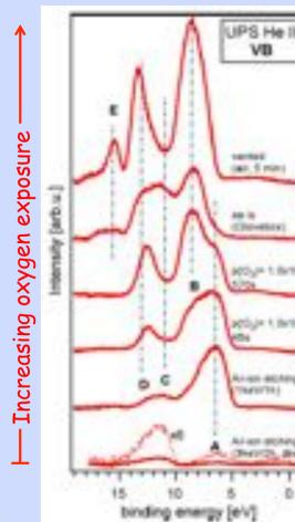
D. Enslin<sup>1</sup> examined lithium surfaces with UPS. Sample was loaded into vacuum under inert atmosphere, cleaned twice via Ar sputtering, and then exposed to two controlled amounts of O<sub>2</sub>. Afterwards, the sample was exposed to air. UP spectra were collected at each stage of the experiment (see figure at left).
