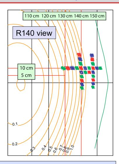
Channel layout provides radial and poloidal correlation lengths and k-spectra
