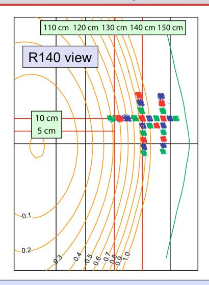
Channel layout will provide radial and poloidal correlation lengths and k-spectra
