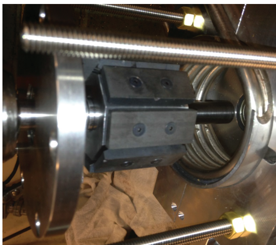
Motor during assembly. 5-turn solenoid of pipe is to the right, magnets are center.
