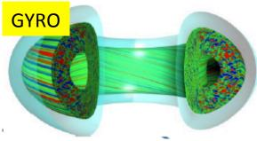
6D Vlasov equations => 5D nonlinear"gyrokinetic"
