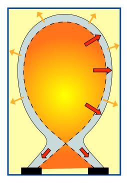
Heat losses from the plasma can damage plasma facing components
