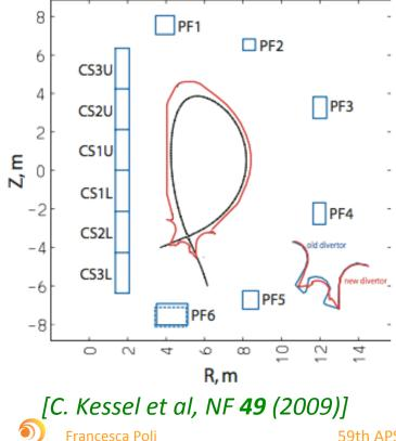
New poloidal field coils layout expands operational space:
