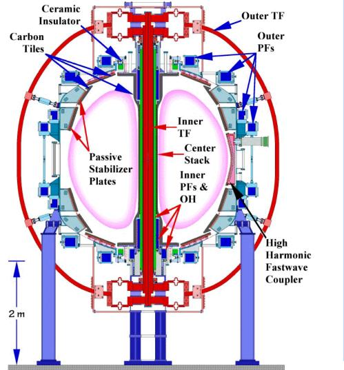
**Baseline Parameter (Achieved)** Aspect Ratio  $\geq$  **1.28** Major Radius = 0.85 m Minor Radius = 0.68 m Elongation = 2.2 (2.5) Triangularity = 0.5 (0.6) Plasma Current = 1 MA (1.4 MA) **Toroidal Field** 0.3 to 0.6 T (≤0.45 T) Heating and CD 5 MW NBI (5.0 MW) 6 MW HHFW (4.2 MW) 0.5 MA CHI (0.26 MA) Pulse Length = 5 sec (0.5 sec)
