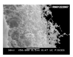
FIG. 1. Foaming of tungsten surface due to bombardment with helium.
