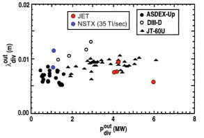
FIG 2. Outer midplane power scrape-off width vs. power delivered to outer divertor.
