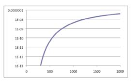
FIG 3. Diffusivity  $(m^2/sec)$  of H in W vs. temperature (K).
