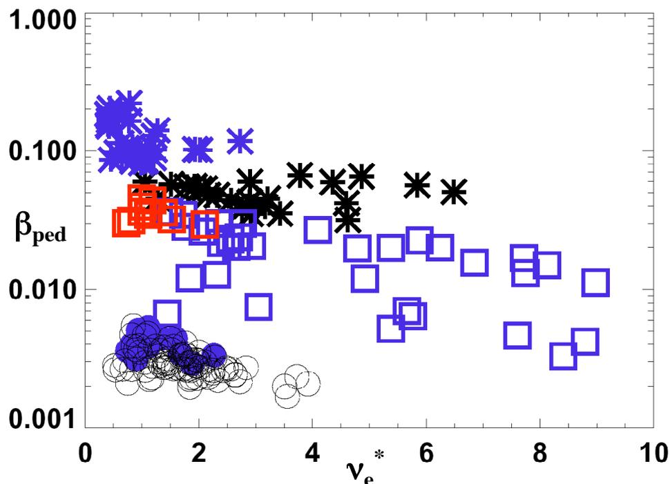
Figure 1: Small ELM edge operational space in Alcator C-Mod (circles), MAST (squares), and NSTX (stars). The color BLACK signifies no small ELMs, BLUE signifies that small ELMs were observed, and RED signifies large ELMs only, i.e. no small ELMs.
