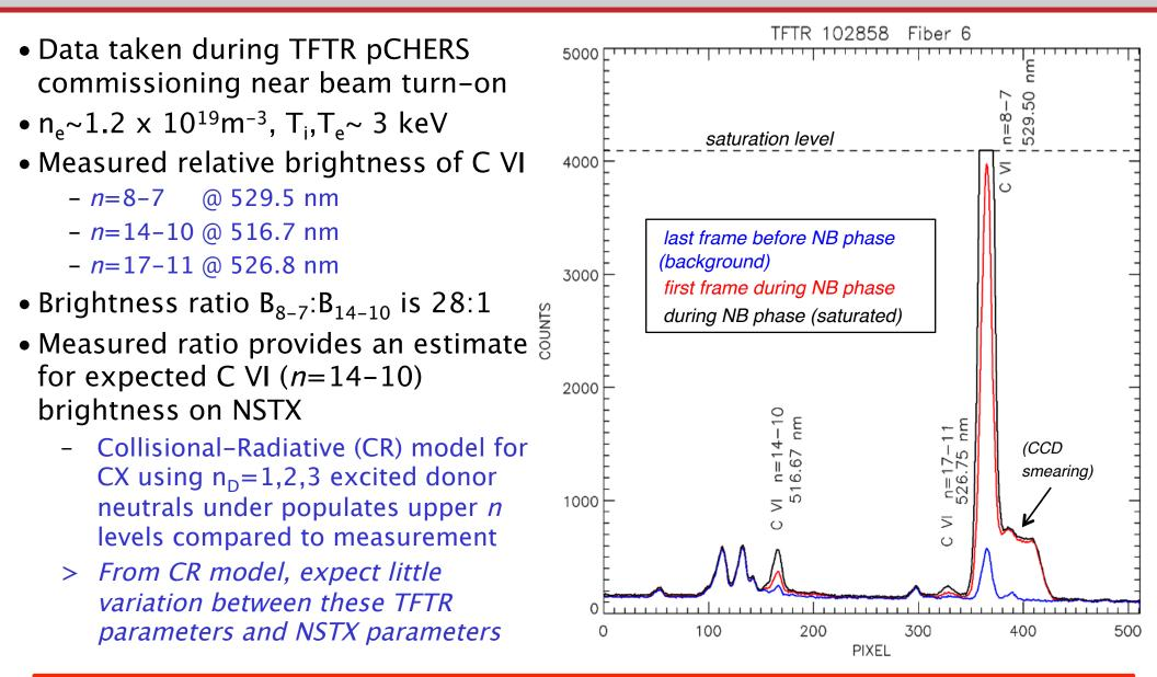
About 50% of brightness @516.7nm on NSTX can be due to C VI
