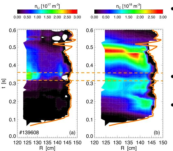
•Large, localized Lithium source can transiently lead to higher n<sub>Li</sub> in the core (as opposed to evaporated lithium or small granules)
