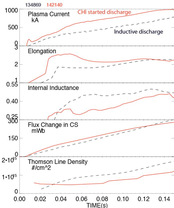
Figure 2: Comparison of time traces for discharges initiated with and without CHI start-up.
