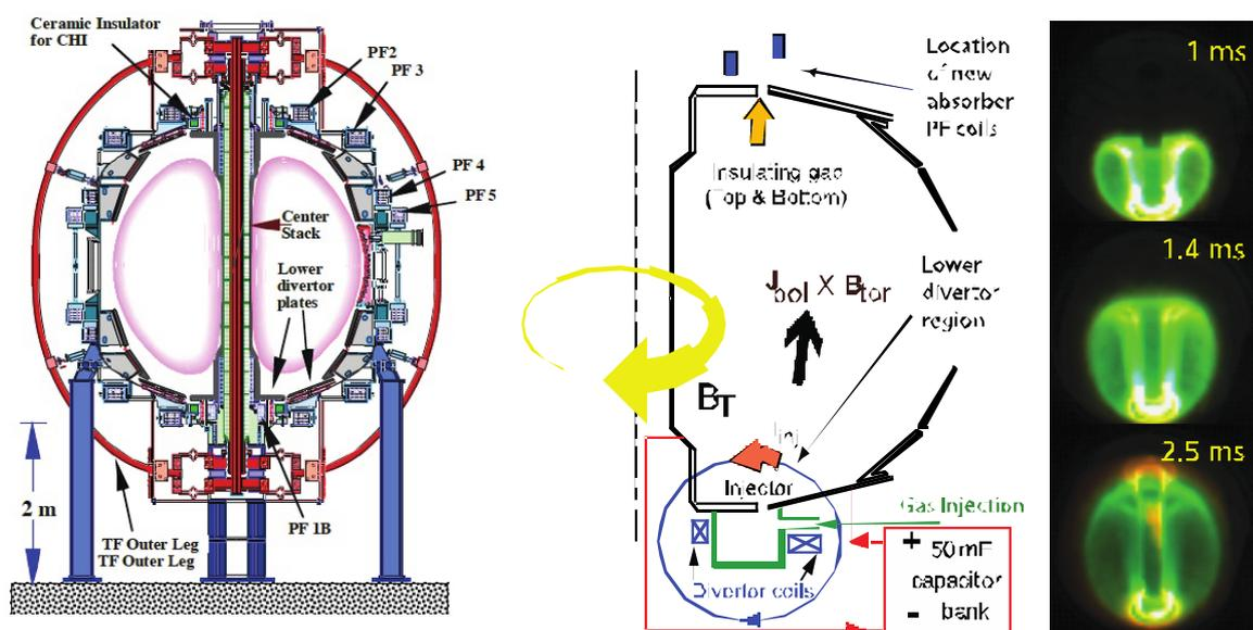
Figure 1: Shown are (left) drawing of the NSTX machine, (middle) cartoon of CHI start-up and (right) fast camera images of an evolving CHI discharge 1ms, 1.4ms and 2.5ms after discharge of the CHI capacitor bank.
