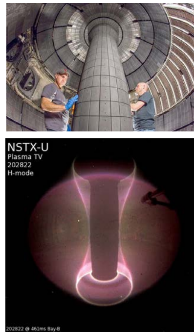
FIG. 1: (top) new NSTX-U centerstack central magnet, (bottom) image of NSTX-U H-mode plasma.
