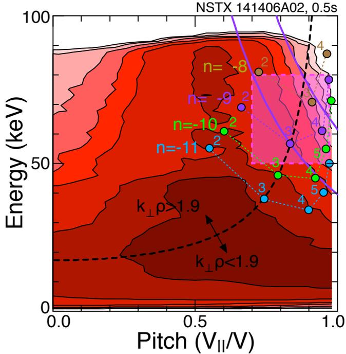
Fig. 3. TRANSP fast-ion distributions for before and after the outboard beam injection. The dashed oval indicates fast ions believed responsible for GAE suppression. Distribution functions are average over whole plasma volume. Contour spacing is linear, beginning at  $1 \times 10^7$  up to  $1.1 \times 10^8$  /  $\text{cm}^3/\text{eV}/\text{dA}$ .
