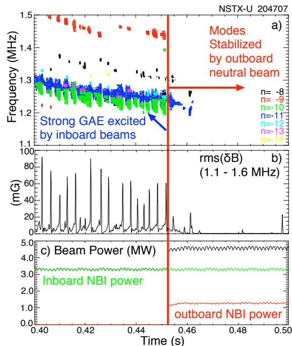
Fig. 1. a) color-coded spectrogram showing GAE activity. Dominant modes are  $n=-10$  (green) and  $n=-11$  (blue). b) RMS magnetic fluctuation amplitude over the frequency range 1.1-1.6 MHz, c) green curve is inboard beam power, red curve is off-axis beam power (source 2c).
