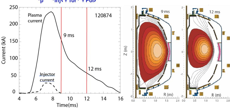
After CHI is OFF, 160kA of non-inductively generated closed flux current is present
