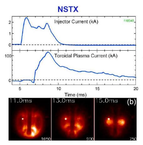
$I_{inj}$  ~1.5 kA generates  $I_p$  ~100 kA - due to Higher Toroidal Flux in NSTX
