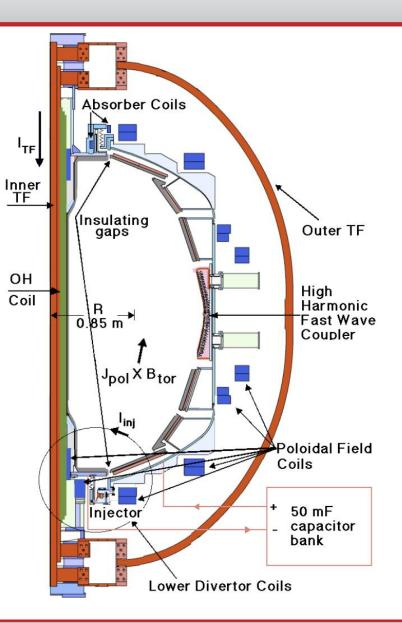
Long-pulse (400ms) CHI discharges in a 'stuffed- injector' current mode used to ablate Low-Z impurities from lower divertor
