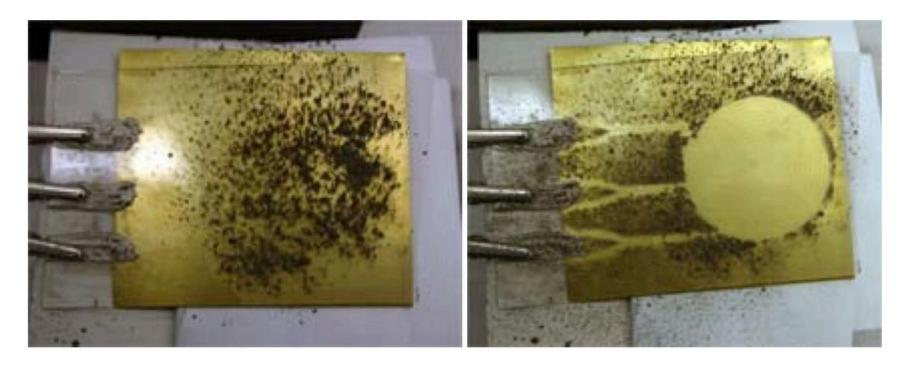
Fig. 4: Before and after photographs of a Dust Shield prototype on a metal plate to provide proof of concept for a sample handling system.
