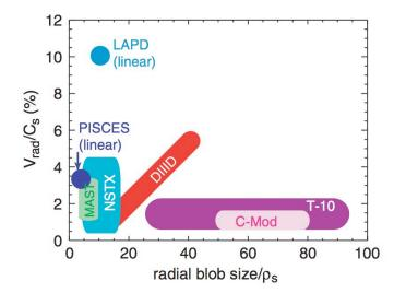
**Figure 3.** Turbulence filament cross-section size and radial velocity in the SOL normalized to the local ion Larmor radius at the electron temperature,  $\rho_s$ , and the local ion sound speed,  $c_s$ , for a number of devices.
