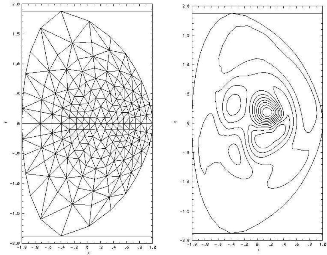
Figure 1: *An example of unstructured mesh and fast ion driven  $n = 1$  mode in a spherical tokamak.*
