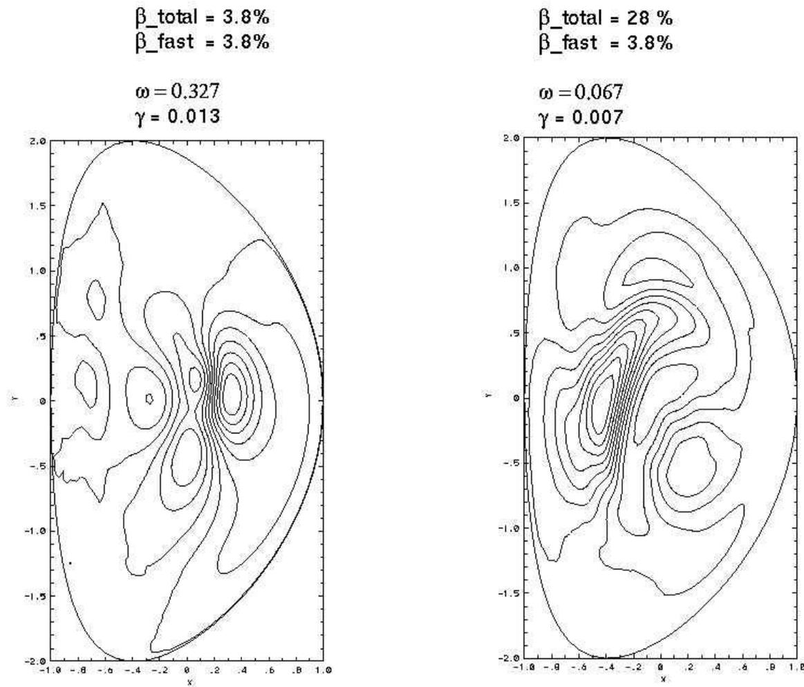
Figure 2: Comparison of fast ion-driven modes at two different plasma beta values.
