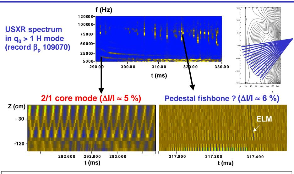
• 300 kHz bandwidth, up to 600 kHz sampling and SNR  $\approx$  100 enable imaging of the low amplitude modes typical of q<sub>0</sub> >1 operation
