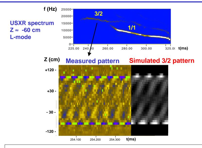
Good match between USXR and EFIT field line trajectory in L-mode
