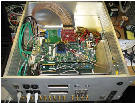
FPGA-based EBW data acquisition and signal processing
