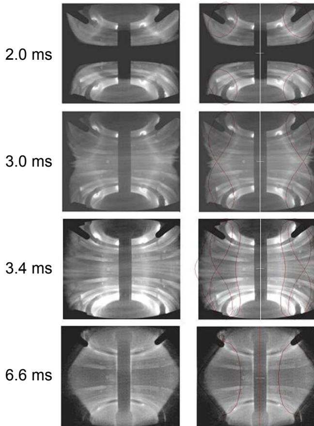
Two plasma rings, inductively formed around P3 in-vessel coils (2.0 ms), merge (3.0 ms), and eventually produce plasma current up to 0.45 MA (6.6 ms).
