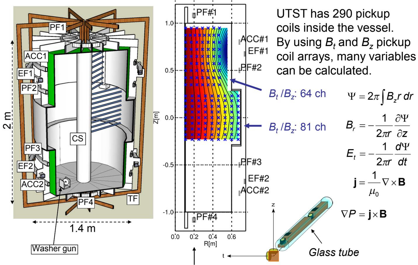
An example of the poloidal flux,  $\Psi$ , of EF.
