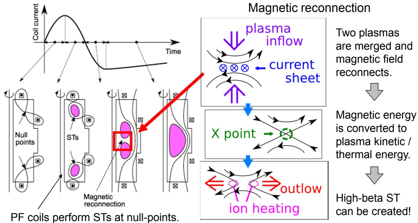
At UTST, DNM start-up is performed by **outer** PF coils to produce a high-beta ST in a reactor relevant situation.
