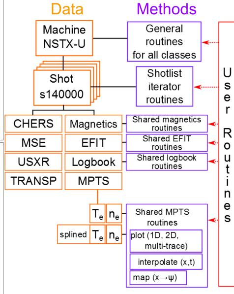
Methods can work at machine, shot, signal group, or signal level
