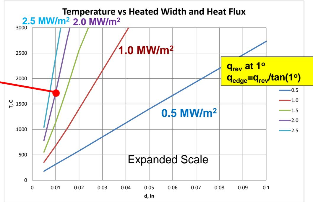
*thermal analysis shows 'enhancement factor' analysis is inaccurate when loading small parts of the tile, so uni-directional shaped tiles can take low reversed heat flux*
