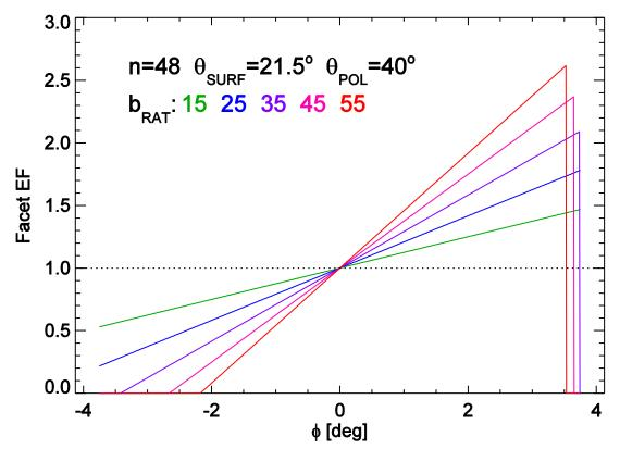
Figure 6: Enhancement for the NSTX-U OBD with  $heta_{pol}=40^o$ , and varying angles of incidence.
