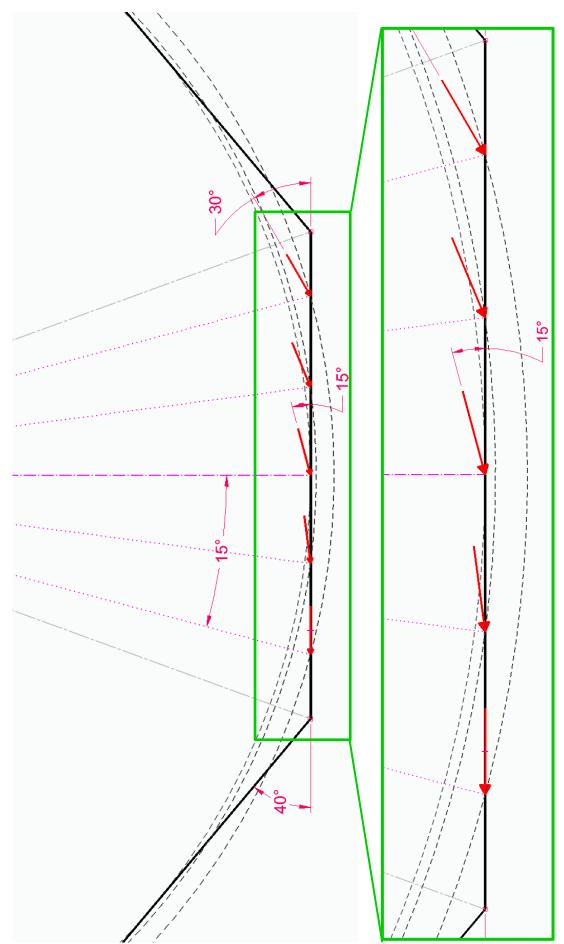
PFFigure 3: Exacerbated, n=9, vertical plate faceted divertor with  $\alpha=15^o$ , highlighting the how) 17 the impact angle changes across the facet and can become tangent, leading to shadowing.
