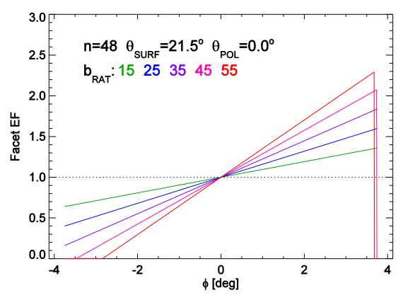
Figure 4: Enhancement for the NSTX-U OBD with  $heta_{pol}=0^o$ , and varying angles of incidence.
