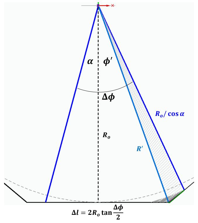
Figure 9: Top down view of faceted, vertical plate divertor for n=9 and  $\alpha=15^{o}$  exacerbating the effect.
