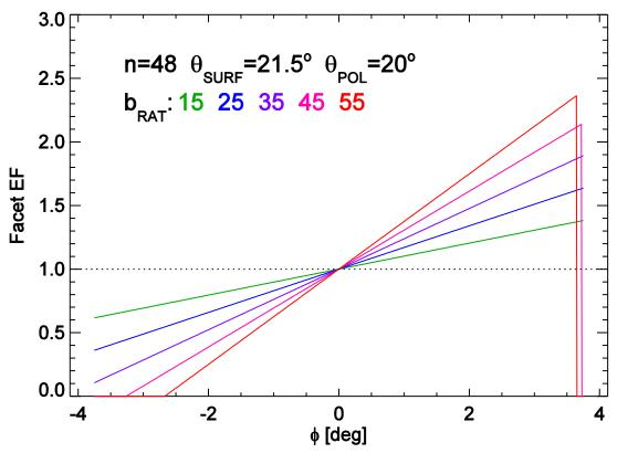
Figure 5: Enhancement for the NSTX-U OBD with  $heta_{pol}=20^o$ , and varying angles of incidence.
