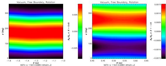
Figure 4—Vacuum Field. The values of  $\delta B_R/B_{\varphi}$  at R = 0.45 m (left) and  $\delta B_Z/B_{\varphi}$  at Z = -1.6 m (right) for the model equilibrium NSTX-U 11613.00851\_NfHz0+\_0, from the TF error field model in the absence of plasma response (i.e. the vacuum field). The inner divertor leg passes through R = 0.45 at Z = -1.477 m, and the outer divertor leg passes through Z = -1.6 m at R = 0.569 m.
