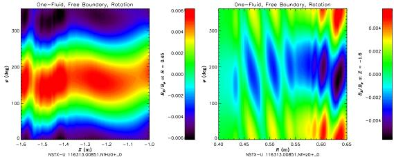
Figure 5—Total Field, Free-Boundary. The values of  $\delta B_R/B_{\varphi}$  at R = 0.45 m (left) and  $\delta B_Z/B_{\varphi}$  at Z = -1.6 m (right) for the model equilibrium NSTX-U 11613.00851\_NfHz0+\_0, from the TF error field, including the plasma response. The inner divertor leg passes through R = 0.45 at Z = -1.477 m, and the outer divertor leg passes through Z = -1.6 m at R = 0.569 m.
