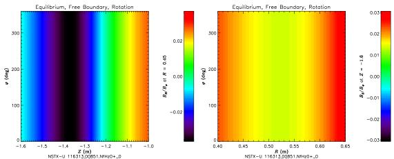
Figure 3—Equilibrium Field. The equilibrium values of  $B_R/B_{\varphi}$  at R = 0.45 m (left) and  $B_Z/B_{\varphi}$  at Z = -1.6 m (right) for the model equilibrium NSTX-U 11613.00851\_NfHz0+\_0. The inner divertor leg
