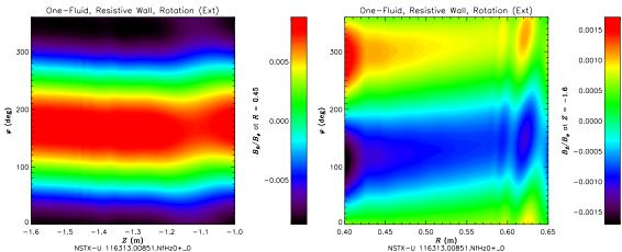
Figure 6—Total Field, Resistive Wall. The values of  $\delta B_R/B_{\varphi}$  at R = 0.45 m (left) and  $\delta B_Z/B_{\varphi}$  at Z = -1.6 m (right) for the model equilibrium NSTX-U 11613.00851\_NfHz0+\_0, from the TF error field model, including the plasma response and the effect of a resistive wall. The inner divertor leg passes through R = 0.45 at Z = -1.477 m, and the outer divertor leg passes through Z = -1.6 m at R = 0.569 m.
