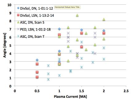
Fig. 4.3.2: Field line angle at the location of peak heat flux versus  $I_p$  for cases in Section 4
