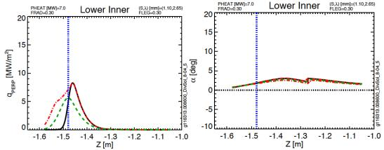
Fig. A.8: Lower inner target parameters from Scan 8-04
