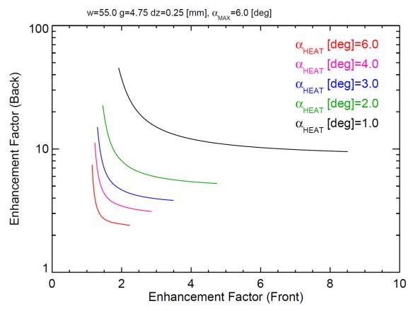
Figure 1: By varying the surface devoted to handling forward directed heat flux compared to reversed field, the heat flux enhancement relative to a conformal flat surface can be derived for both the front facing and back facing surfaces.
