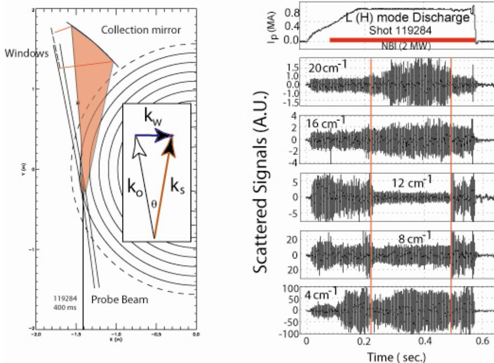
Fig. 2. Scattered raw signal at five different wave-numbers from NBI heated plasmas where L/H transition and corresponding changes in scattered power spectra are clear.
