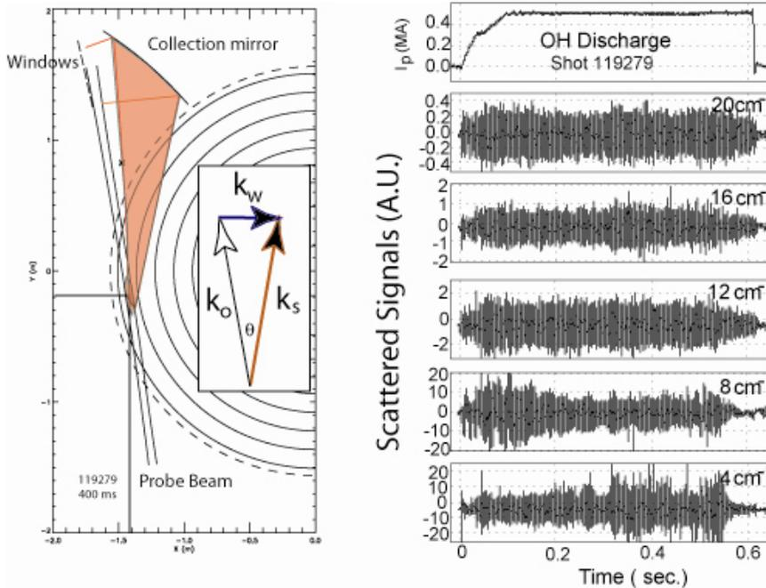
Fig. 1. Scattered geometry and raw scattered signals at five different wavenumbers of the OH discharge.
