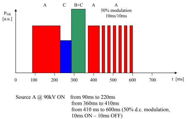
Desired waveform for NB power:
