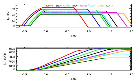
Figure #2: Example TF waveforms, along with their approach to the I<sup>2</sup>t limit of the coil.
