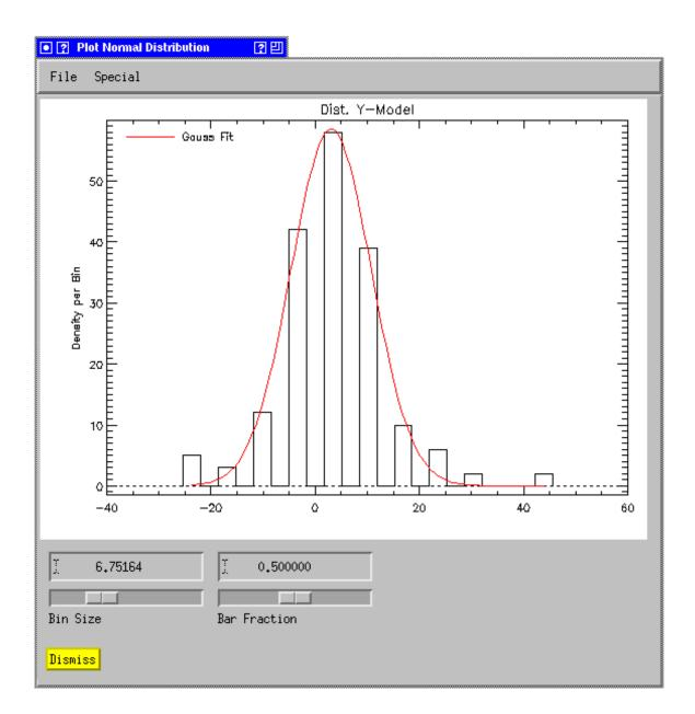
You can create this plot for individual parameters by clicking on a parameter in the "DbAccess Model" window, and clicking the "<-Plot Distribution" button.
