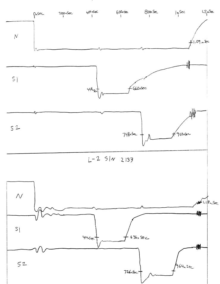
3952 Crate controller timing diagrams referencing 51,52, and the time The L-2 takes data to the leading edge of the "N" line in skt 10.
