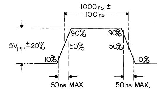
FIG IO.I STANDARD TIMING PULSE
