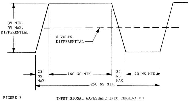
FIGURE 3 INPUT SIGNAL WAVESHAPE INTO TERMINATED
