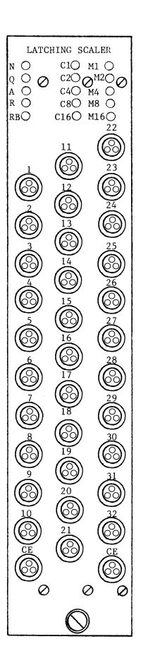
Suggested front panel layout  $\label{eq:figure 1} \mbox{Figure 1}$
