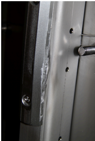
Melted moly limiter
