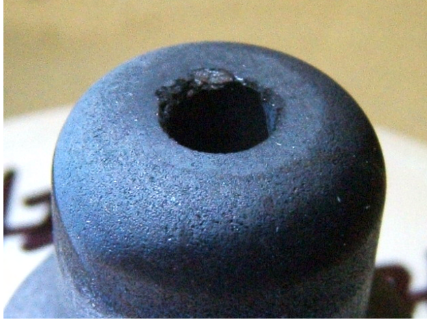
Fig. 15. A photograph of the SGI nozzle eroded by plasma after six years of operation.
