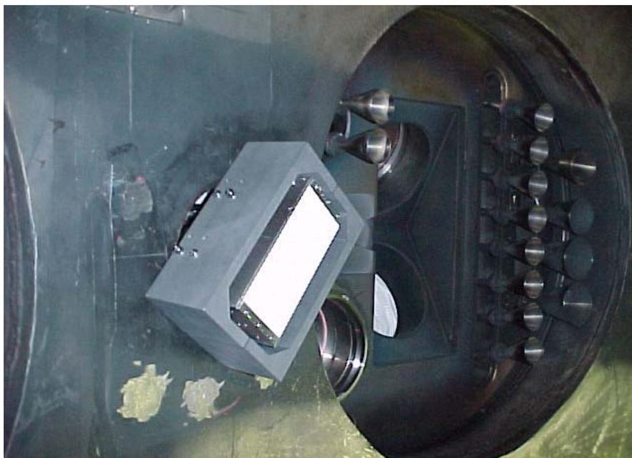
*Fig. 2.19 Dual-horn EBW receiver/edge reflectometer (behind the white boron nitride shield) with movable graphite limiters in NSTX*
