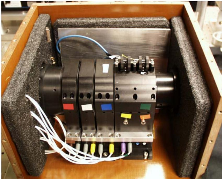
Fig. 2.18 Tunable Lyot filter and detector housing for MSE/CIF system
