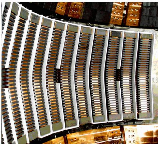
Figure 3.3.1 The twelve-strap HHFW antenna array.
