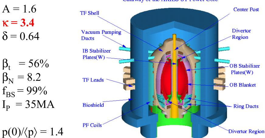
Cutaway of the ARIES-ST Power Core
