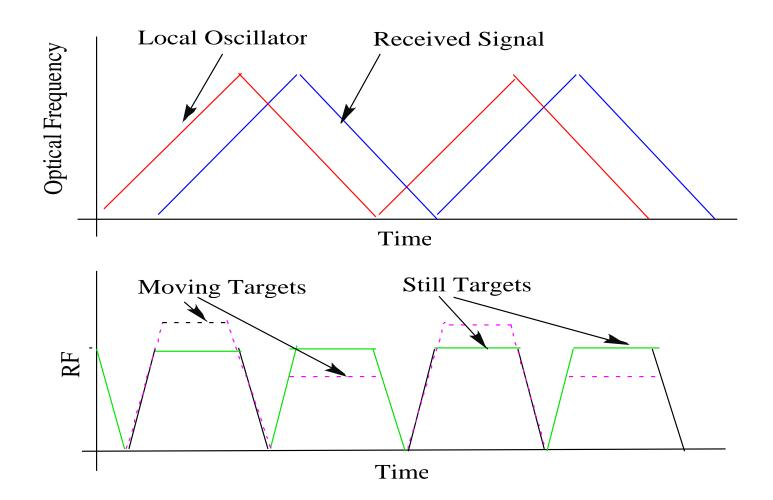
Symmetric up-shift/down-shift modulation permits Doppler corrected range and velocity measurements.
