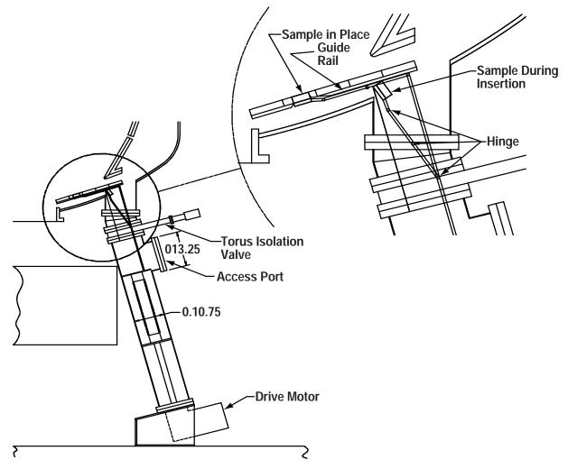
Schematic of the NSTX-DiMES sample changer system concept (an example)
