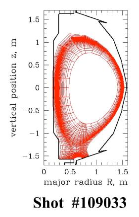
In the Lower Single Null magnetic configuration, the surface area connected to the inboard SOL is much ( $\sim$ 10X) smaller than the area connected to the outboard SOL.
