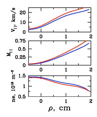
Here magnetic flux surfaces are mapped to the outboard mid-plane. The inner SOL is ~2.5X broader. At the inner mid-plane, plasma in over entire width of SOL moves down toward the inner divertor plate.
