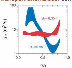
Low-k microtearing important in "Hybrid" and weak RS discharges Inferred  $\chi_\epsilon$  agrees with predictions from non-linear theory
