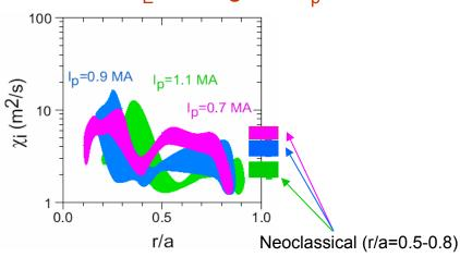
Neoclassical levels determined from GTC-Neo: includes finite banana width effects (non-local)
