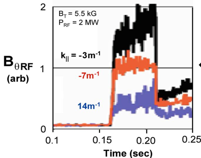
HHFW at low  $k_{\parallel}$  should begin propagating at much lower  $n_e \rightarrow$  surface waves, wall interactions
