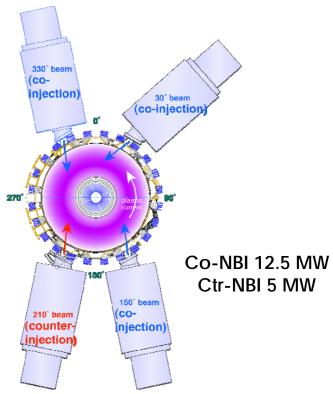
NSTX has also used unbalanced NBI perturbation for core pinch studies  On both NSTX and DIII-D, n=3 non-resonant magnetic fields
