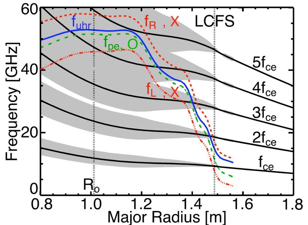
EBW emission data can be used to provide coupling efficiency and polarization information for heating and current drive system
