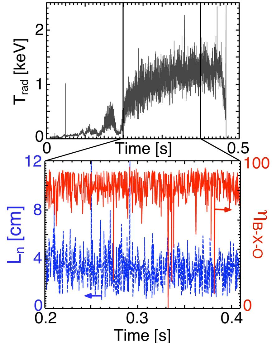
Maximum  $T_{\text{rad}}$  used to calculate measured  $\eta_{\text{B-X-O}}$
