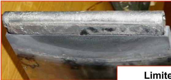
Limiter from Mo mesh with pore size of 75 \mu\text{m}
