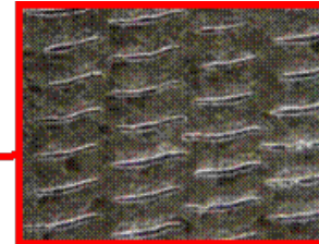
View of limiter surface after 2000 plasma shots
