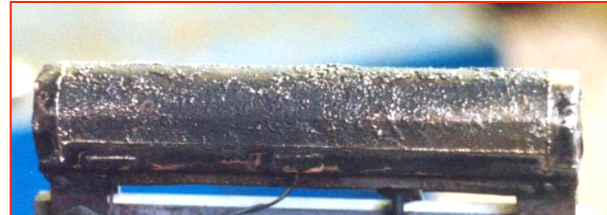
Limiters from SS mesh with pore size of 15 -50 \mu\text{m}
