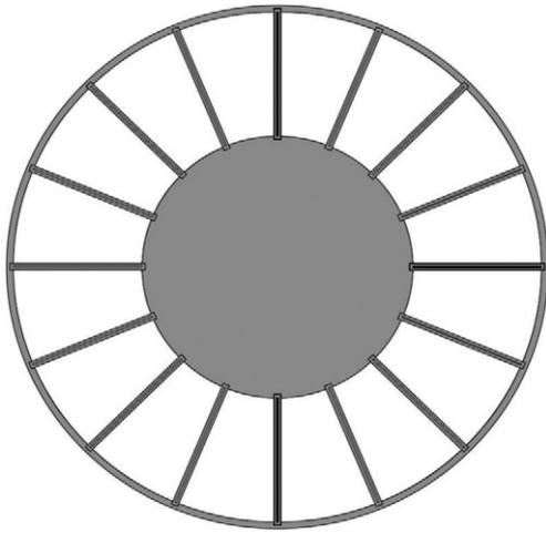
**Fig. 1.** Horizontal cross-section view of the center portion of the all-metal center stack. The central region is ferritic material, surrounded by copper wedges, which are in turn separated by resistive inserts.
