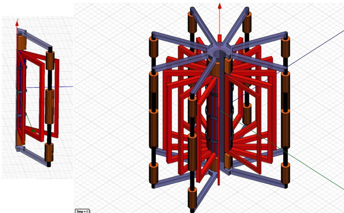
**Fig. 2.** (a) Single (1/8) sector of the model. The copper TF coil is shown in red, iron in purple, Inconel is in blue. The superconducting coils that drive the system are in orange. (b) A 3/4 sector of the same model for visualization. (For interpretation of the references to color in this figure legend, the reader is referred to the web version of the article.)
