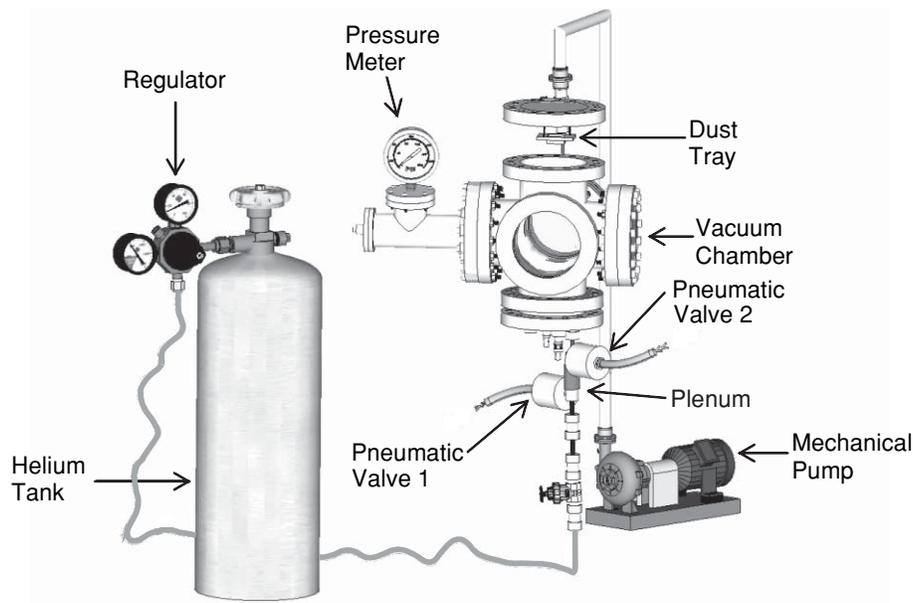
FIG. 1. Setup used for He puffs in vacuum. The upper flange is raised to show the dust delivery tray.
