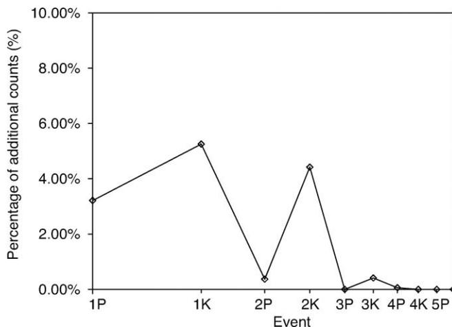
FIG. 4. Percentage of additional counts triggered by consecutive puffs labeled 1P, 2P, 3P, . . . and knocks labeled 1K, 2K, 3K, . . . in vacuum conditions with the cover mesh and four-nozzle manifold. After two puffs an insignificant number of additional counts were triggered by a knock event indicating that the entire surface of the detector was cleared.
