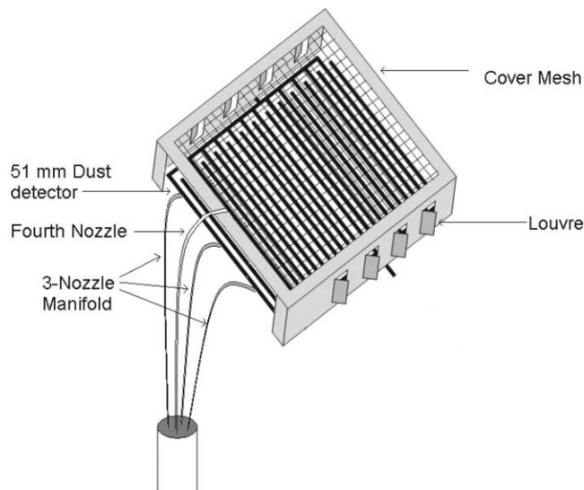
FIG. 3. Puff system setup with the 5 cm  $\times$  5 cm dust detector and cover mesh as used previously in NSTX (Refs. 4 and 5). The detector is shown schematically by the thick lines under the cover mesh. For clarity the mesh porosity is not to scale. Three of the nozzles are aimed on the surface of the detector and the fourth nozzle is aimed at the surface of the mesh.
