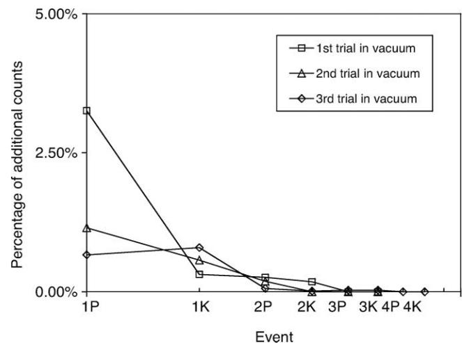
FIG. 2. Percentage of additional counts triggered by consecutive puffs labeled 1P, 2P, 3P, ... and knocks labeled 1K, 2K, 3K, ... in vacuum conditions without cover mesh and with the three-nozzle manifold. For three trials the percentage of additional counts triggered by a knock event after a second puff was lower than 0.5%.
