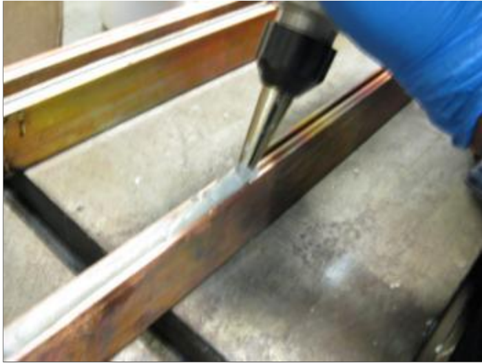
Solder paste injection over cooling tube
