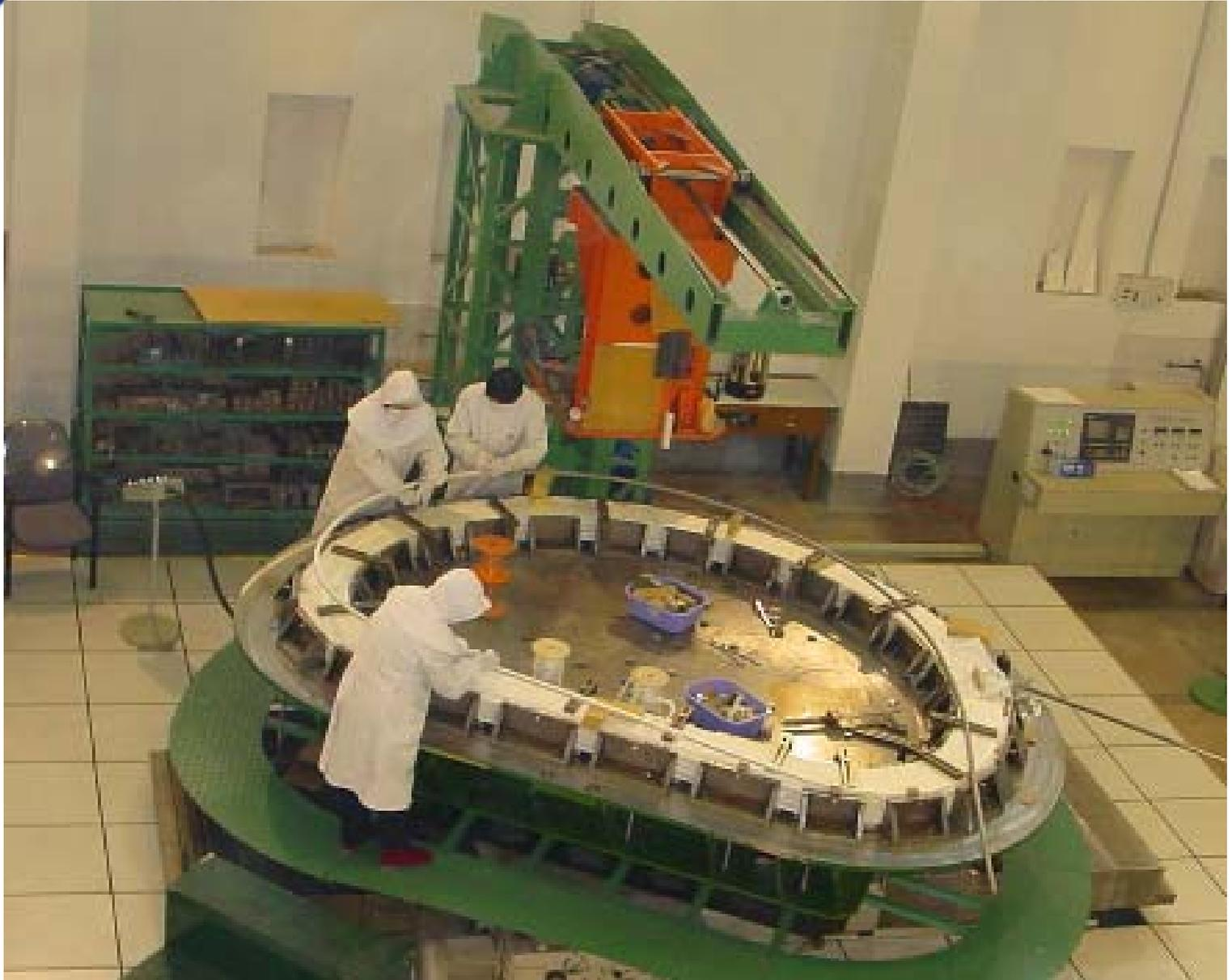
TF prototype coil winding
