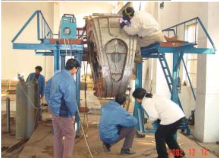
**Thermal Shield fabrication**
