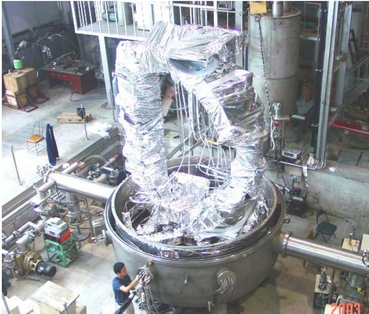
**TF prototype coil in test facility**
