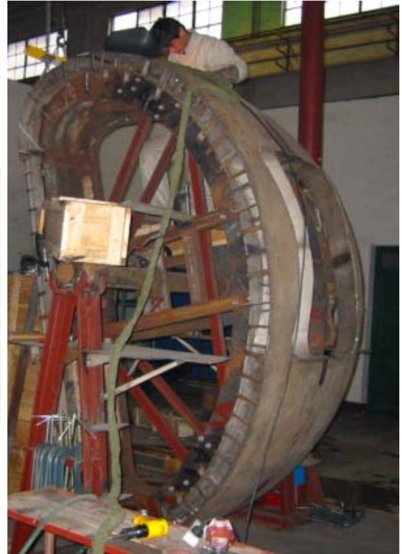
**Prototype of Vacuum Vessel
