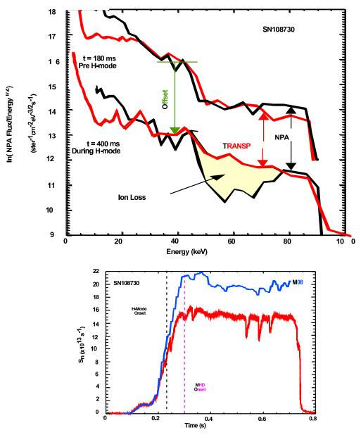
Figure 5. The TRANSP code is capable of simulating the NPA flux measurements. The measured and simulated energetic ion spectra are compared for times t = 180 ms
