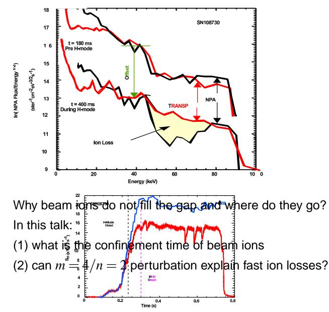
Figure 5. The TRANSP code is capable of simulating the NPA flux measurements. The measured and simulated energetic ion spectra are compared for times t = 180 ms
