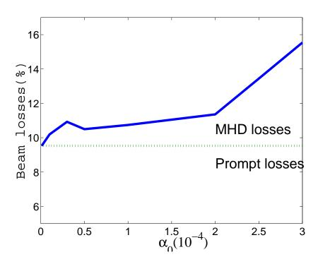
At expected amplitudes  $\alpha_0 = 2 - 3 \times 10^{-4} (\delta B/B) \sim 10^{-3}$ , m = 4/n = 2 mode can induce losses comparable to prompt losses.
