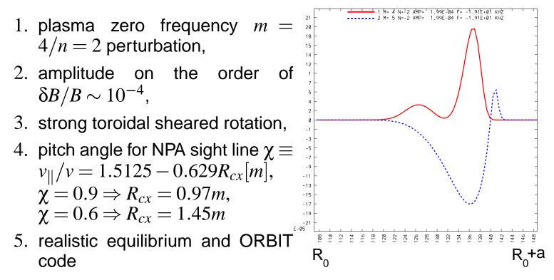
mode structure consistent with ideal MHD  $\delta \mathbf{B} = \nabla \times \alpha \mathbf{B}$  $\alpha \sim (1 - nq/m) (r/r_s)^m \sin(n\varphi - m\theta)$ , if  $r < r_s$
