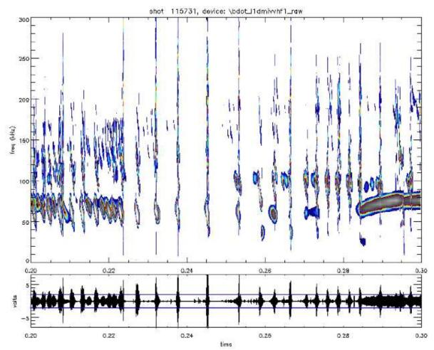
At t=0.262sec, n=2 mode frequency  $f_{lab}\simeq 103\,kHz$ ,  $f_{pl}\simeq f_{lab}-n\times 30=43\,kHz$ ,  $\Rightarrow$  too low for TAE for all observed modes.
